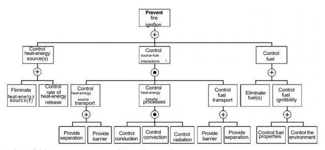
FIGURE G.3.6(b) Example Prevention of Fire Ignition Flow Chart.
