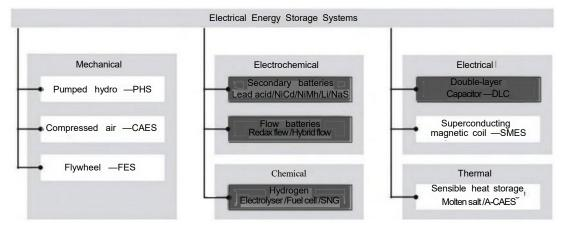
FIGURE D.1 Classification of Electrical ESS.(Source:Fraunhofer ISE.)
