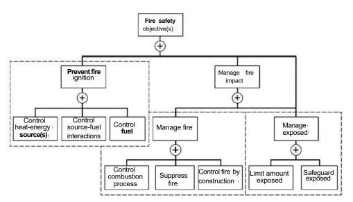
FIGURE G.3.6(a) Example Fire Safety Objectives Flow Chart.
