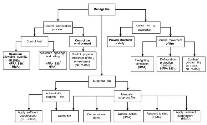
FIGURE G.3.6(e) Example Manage Fire Flow Chart.
